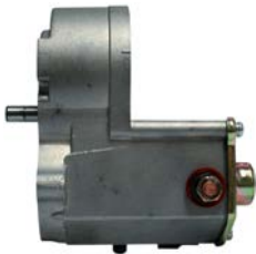
236596 Solenoid Assy Servicing: 03101-3170 12 V, No./ terminals 3
