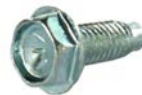
233408 Screw Replacing: 387448-s100, 383338-s2 Servicing: 5MT, 10MT, D80F11001AA, E1AF11001BA Thread length 1/2", Total length 41.00/64", Thread 10.32 Hex washer head 5/16" drive w/ serrated flange.
