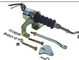
090096 Solenoid Shutdown Kit Replacing: sa-3799-12 12 V, 1.1 A/ hold, 46 A/ pull, Hold rating 178N, Pull rating 89N at 25.40 mm, Elect. connection Cable, Function Pull This solenoid can't switch off by itself, it will have to be controlled externally.
