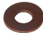
234294# Brake Washer Replacing: sz628, CODZ11036A Servicing: c7af11001b, D80F11001AA, e1af11001ba ID 15.88, OD 34.93, Thickness 3.20, Material Fiber
