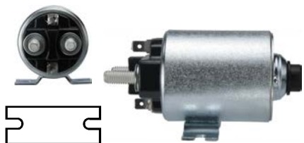
333009 Solenoid 12 V, 150 A, OD 52.20, Coil bolt M8, No./ terminals 4
