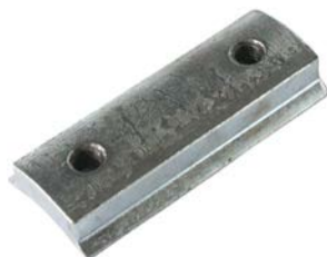
234505 Pole Shoe Servicing: 0001364400 Length 100.30, Height 15.80, Width 41.65, Thread size M10
