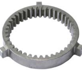
235173 Gear Wheel Servicing: 0001107072, 0001121008, 0001121009, 0001121010, 0001121011, 0001121016, 0001121017, 0001121026, 0001121027, B001120046 ID 48.50, OD 58.00, Height 10.00, No./ teeth 40
