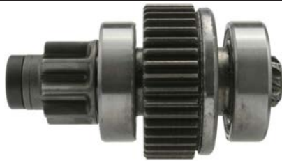
236607 Drive Servicing: 03101-3170, 03101-3190, 03101-3220 OD 29.00, Total length 93.50, Rotation CR, No./ teeth 9, Splines A 10
