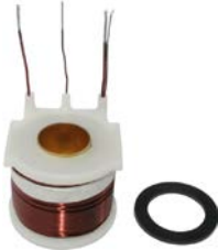
138934 Solenoid Coil 12 V, ID 21.00, OD 46.55
