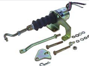
090095 Solenoid Shutdown Kit Replacing: sa-3742-12 12 V, 1.1 A/ hold, 46 A/ pull, Hold rating 178N, Pull rating 89N at 25.40 mm, Elect. connection Cable, Function Pull This solenoid can't switch off by itself, it will have to be controlled externally.
