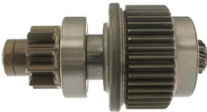
235095 Drive Servicing: 03111-4140, 03111-4240, 03111-4241 OD 32.00, Total length 104.00, No./ teeth 10, Splines A 10
