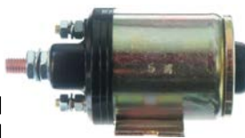
133695 Solenoid Replacing: cey113, 099845 12 V, 100 A, Intermittent load 500 Amp., OD 47.70, Coil bolt M8, Seconds 5, No./ terminals 4
