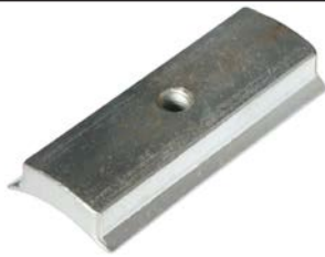
234197 Pole Shoe Length 99.60, Height 15.75, Width 41.15, Thread size M10
