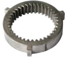
234919 Gear Wheel Servicing: 1006200101 ID 46.40, OD 62.30, Height 13.30, No./ teeth 37
